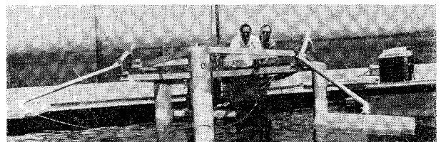
Fig. 3 Prototype shown with hydrofoils retracted.
